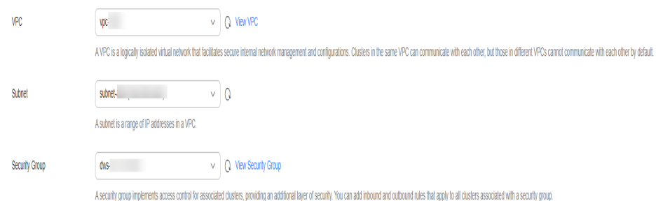
Figure 3-3 Configuring network specifications
